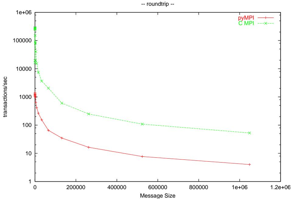
Figure 10: Ping-pong test in C MPI and pyMPI
