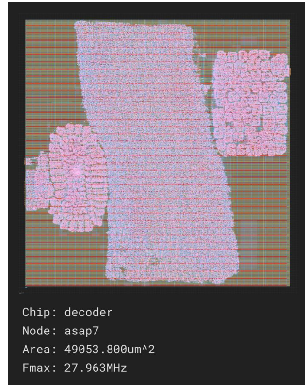
Decoder ASIC generated by Siliconcompiler
