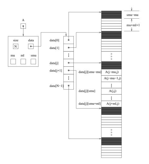
Figure 8.1: Diagram of the storage for the SUNMATRIX\_BAND module. Here A is an  $N \times N$  band matrix with upper and lower half-bandwidths mu and ml, respectively. The rows and columns of A are numbered from 0 to N - 1 and the (i, j)-th element of A is denoted A(i,j). The greyed out areas of the underlying component storage are used by the associated SUNLINSOL\_BAND linear solver.
