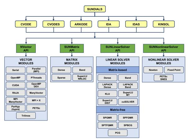
Figure 3.1: High-level diagram of the SUNDIALS suite.
