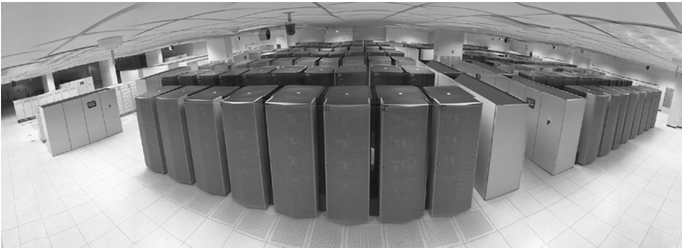
Figure 19. ASCI White (2001), featuring 12.3 teraflops peak performance.
