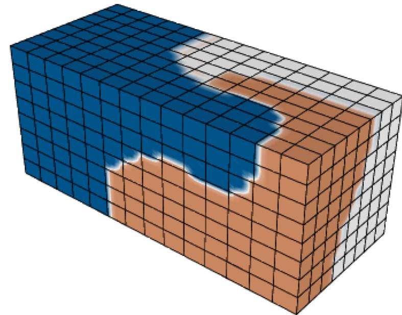
3D triple point problem on a static mesh and on a moving mesh with Lagrangian framework.
