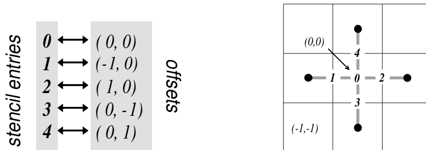
Figure 2.4: Representation of the 5-point discretization stencil for the example problem.
