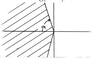
All the BDFs up to order 6 are "Stiffly Stable": A.S.R. includes a half-plane left of some d < 0, and method is accurate in an adjoining rectangle centered at the origin.
