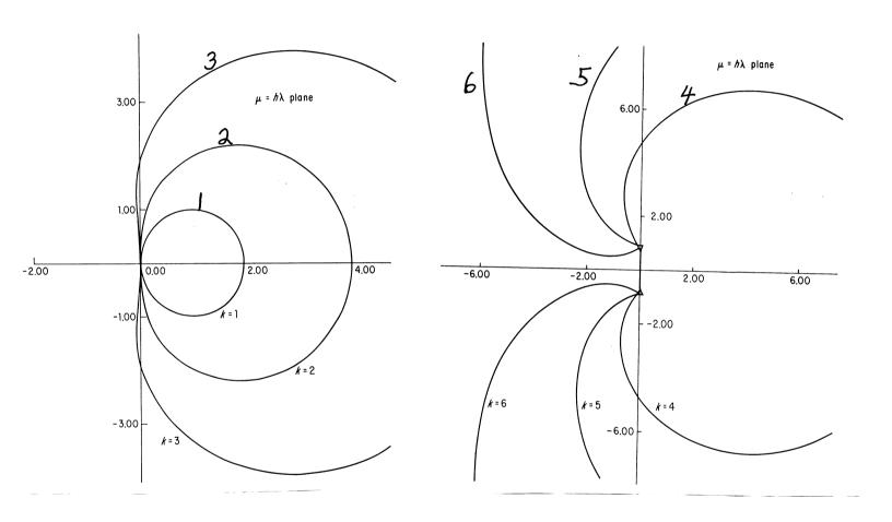
Order 6 is close to failing to be  $A(\alpha)$ -Stable or stiffly stable, so is excluded in the BDF solvers.
