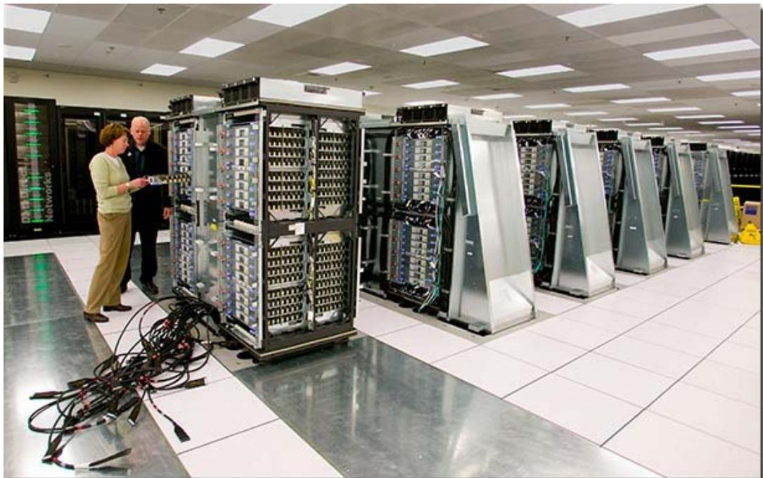
Kim Cupps, LLNL High Performance Systems Division leader, and Mark Seager, LLNL assistant department head for New Technologies, inspect a newly installed rack for Dawn, a 500 teraFLOP/s (trillion floating operations per second) IBM BlueGene/P system. Dawn will help lay the foundation for the 20 petaFLOP/s (quadrillion floating operations per second) Sequoia system.
